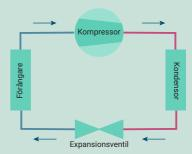
Simple schematic of the refrigeration cycle. The compressor, condenser, expansion valve and evaporator work together to move heat – this is how cooling is created and why heat can be recovered in the process.
